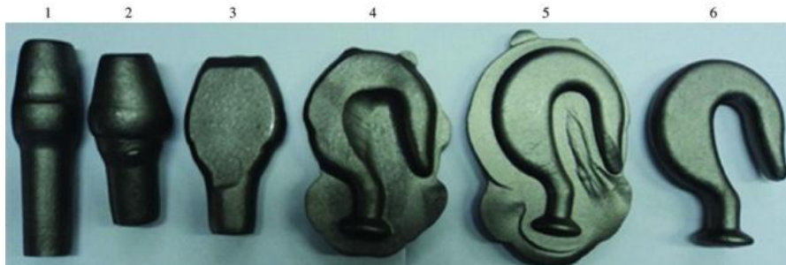
Figure 2. Workpieces during forging stages 1-6 (from left to right): 1-2: upsetting; 3: flattening; 4-5: die-forging; 6 final product after flash removal [21].
